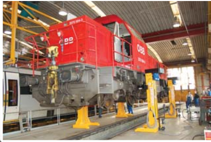
Lifts for Locomotives
